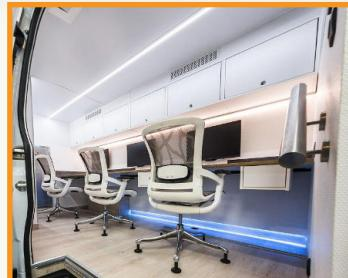
Completely independent energy supply and management system with sophisticated sound and heat insulation. Special AC unit with improved climate control for hot regions and high humidity.
