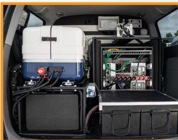
Completely independent energy supply system and UPS with up to 10 hour battery backup. Generator provides power for 99 hours independent use with special silent mode. Our worldwide unique Swing Rack enables the long-term secure operation of IT equipment and servers in a moving vehicle.
